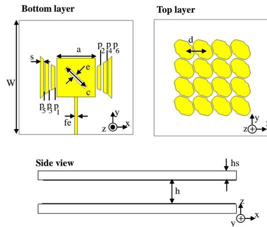
Fig. 3. Structure of element antenna using the proposed metasurface ( $a = 10.5$ ,  $c = 7.5$ ,  $d = 5$ ,  $e = 1$ ,  $fe = 0.7$ ,  $g_1 = 0.5$ ,  $g_2 = 0.7$ ,  $g_3 = 0.3$ ,  $h = 4$ ,  $hs = 1.6$ ,  $p_1 = 5$ ,  $p_2 = 7$ ,  $p_3 = 8$ ,  $p_4 = 9$ ,  $p_5 = 9.5$ ,  $p_6 = 11.5$ ,  $s = 1$ ,  $W = 33$ ) Unit: mm.
