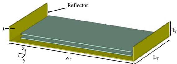
Fig. 16. The  $2 \times 4$  array antenna with the reflector.
