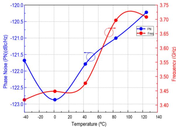
Fig. 12. Simulated PN and frequency across temperature from -40 °C to 125 °C.
