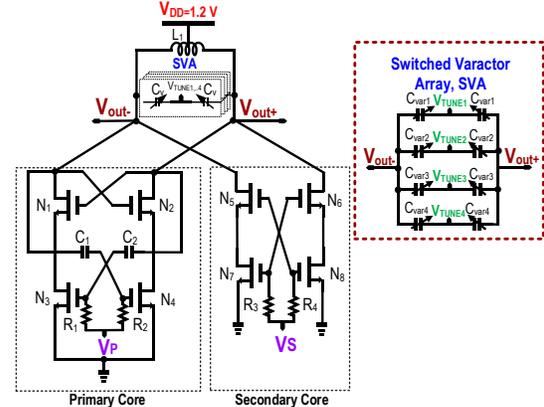
Fig. 2. Proposed LC-VCO with dual core VCO.
