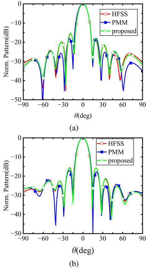
Fig. 4. The normalized 2D radiating pattern of 64-element 2-D planar array in different methods, (a)  $xoz$ -plane, (b)  $yozy$ -plane.
