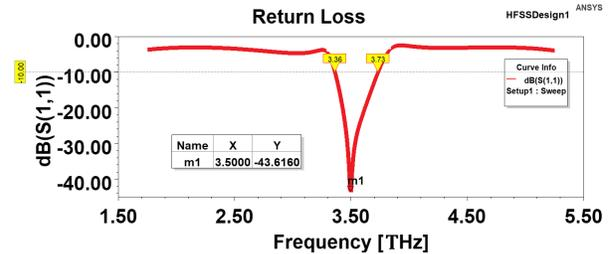
Fig. 4. Simulated return loss value at 3.5 THz.
