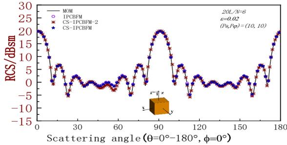
Fig. 5. HH polarization monostatic RCS of the cube.
