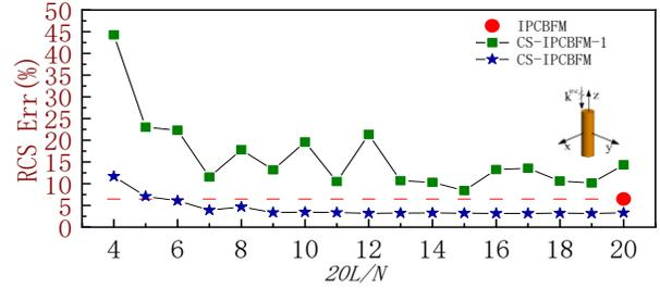
Fig. 4. RCS Err of the cylinder for different  $L$ .
