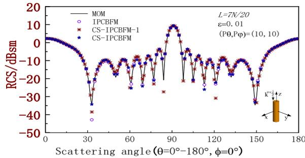
Fig. 1. HH polarization monostatic RCS of cylinder.
