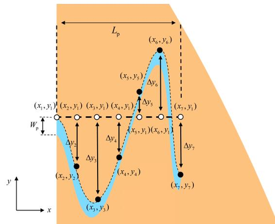
Fig. 2. Diagram of the parametric modeling for curves.
