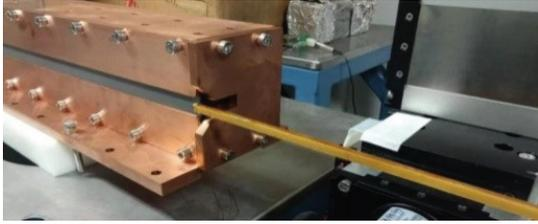
Fig. 9. Point coil for measuring the end field.
