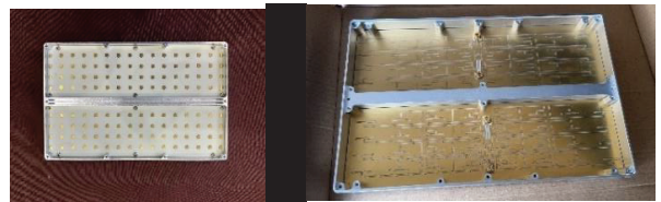
Fig. 9. Photograph of the fabricated antenna in Fig. 1.
