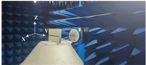
Fig. 10. Photograph of measuring the fabricated antenna in Fig. 1.
