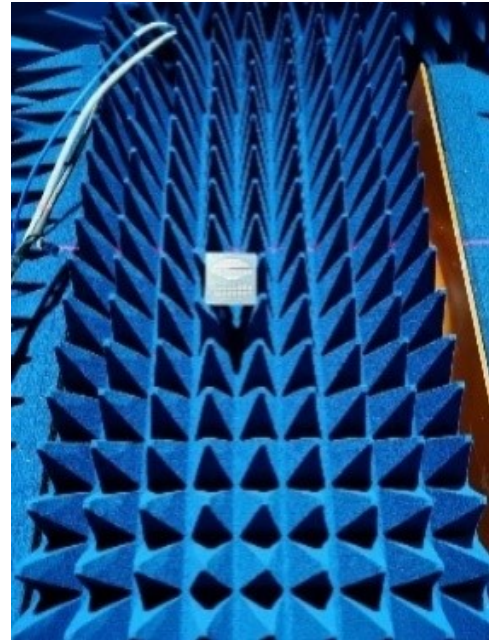
Fig. 7. Measurement setup of the bowtie antenna TRM.
