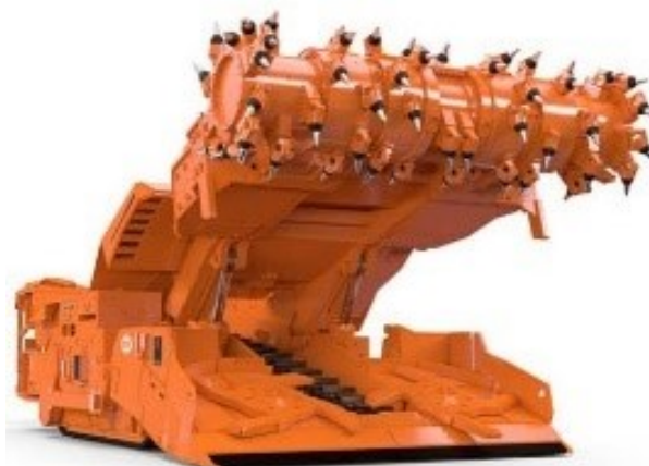
Fig. 1. Picture of a continuous miner commonly used in mining of coal, trona, salt and soft rock types. Pick cutters are mounted on a drum to apply force and break the rock [14].
