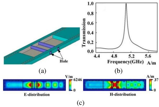
Fig. 3. (a) Structural diagram of a two-channel sensor (the upper metal is hidden), (b) transmission coefficients  $S_{21}$ , and (c) electric field distribution and magnetic field distribution at 5.1 GHz.
