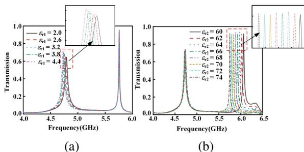
Fig. 5. (a) Transmission coefficients corresponding to the relative permittivity of different polyimide materials and (b) transmission coefficients corresponding to the relative permittivity of different distilled waters.
