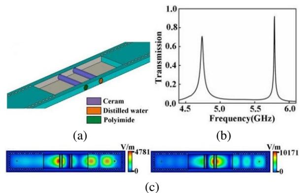
Fig. 4. (a) Dual-channel sensor loaded with polyimide material and distilled water, (b) transmission coefficients  $S_{21}$ , and (c) electric field distribution maps corresponding to 4.74 GHz and 5.75 GHz.
