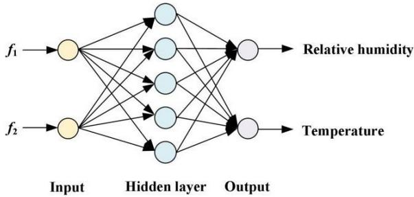
Fig. 7. Structural diagram of BP neural network.
