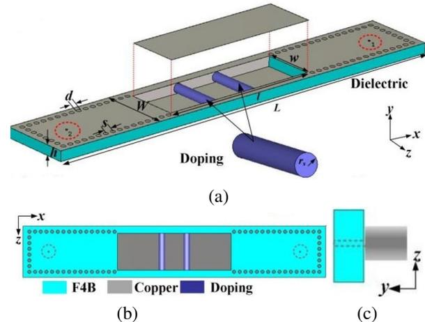
Fig. 1. (a) Structural diagram, (b) top view, and (c) side view of double-doped CPNZ media sensor.
