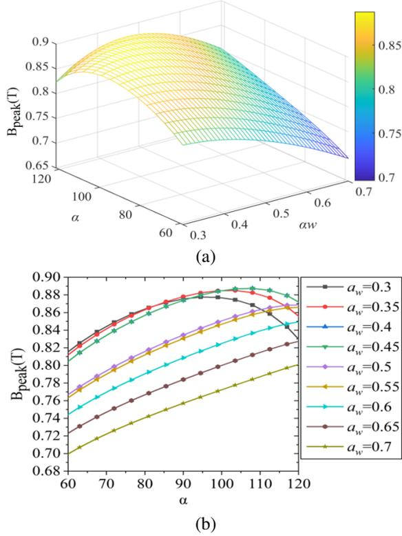
Fig. 9. The effect of  $a$  and  $a_w$  on  $B_{\text{peak}}$  ( $a_h = 0.5$ ,  $a_g = 0.5$ ): (a) three-dimensional topography of  $B_{\text{peak}}$  with  $a$  and  $a_w$  as variables and (b) analysis of influence law of  $a$  and  $a_w$  on  $B_{\text{peak}}$ .
