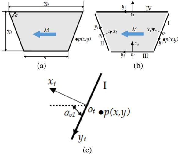
Fig. 4. Schematic diagram of  $-x$  magnetization coordinate rotation: (a) horizontal left magnetization, (b) relative coordinate system established by side length, and (c) angle  $\alpha_{v1}$  between side I and the magnetizing direction.
