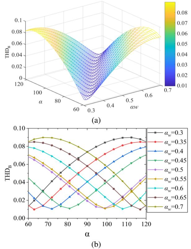
Fig. 7. The effect of  $a$  and  $a_w$  on  $\text{THD}_B$  ( $a_h = 0.5$ ,  $a_g = 0.5$ ): (a) three-dimensional topography of  $\text{THD}_B$  with  $a$  and  $a_w$  as variables and (b) analysis of influence law of  $a$  and  $a_w$  on  $\text{THD}_B$ .
