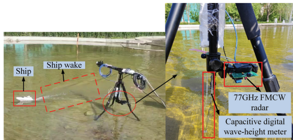
Fig. 10. Experimental setup for measuring ship wake wave heights in a water pool.
