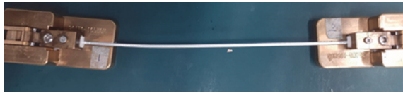
Fig. 24. Device for 100-ohm cable measurement.
