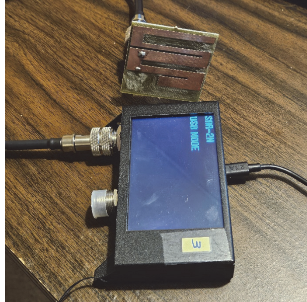
Fig. 7. Test configuration of the sensor antenna using NanoVNA v2 and a host computer.
