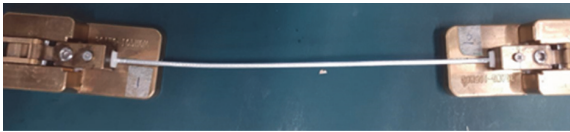
Fig. 24. Device for 100-ohm cable measurement.
