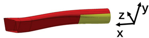
Fig. 13. Partial coating scheme for cavity in Fig. 12 (red area is coated).
