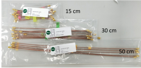
Fig. 2. Coaxial cables used for measurement.
