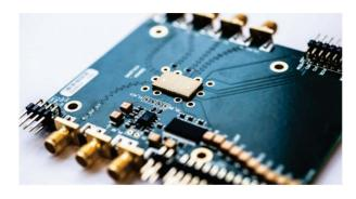
Fig. 2. 60 GHz mmWave radar. Adapted from [3].
