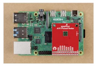
Fig. 4. A111 HAT v1.1 and v1.0 stacked on a Raspberry Pi. Adapted from [8].
