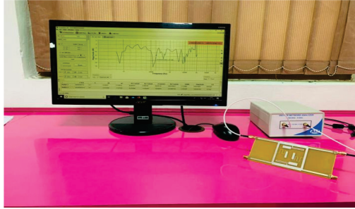
Fig. 14. Experimental setup for DBBLC.
