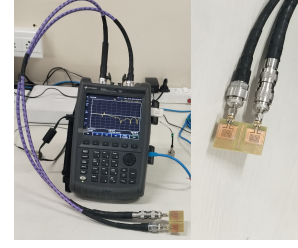
Fig. 6. Photograph of the fabricated antenna and measurement setup of the proposed MIMO antenna.
