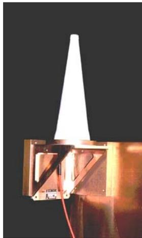
Fig. 6. Pyramidal antenna placed onboard the satellite.
