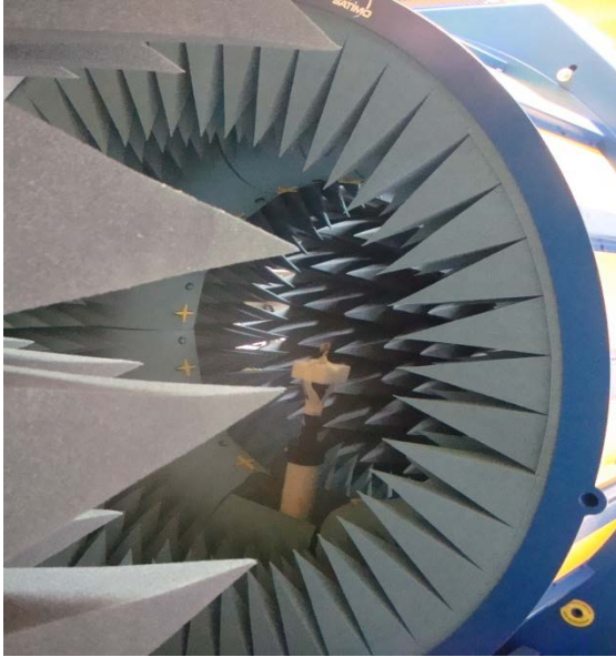
Fig. 7. Antenna measurement setup in StarLab.
