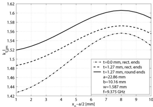
Fig. 2. Normalized resonant length versus slot offset.
