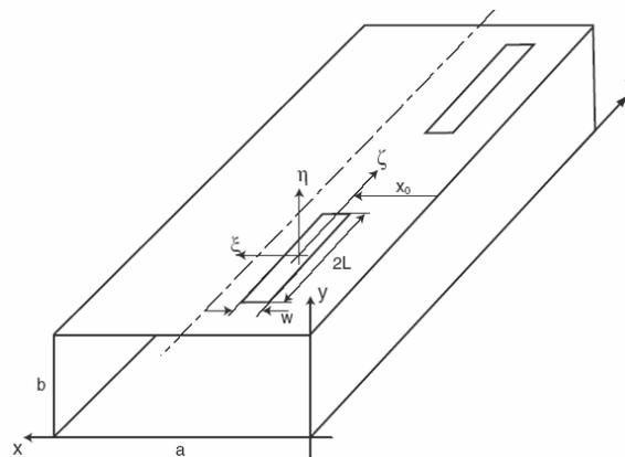
Fig. 1. Longitudinal slots cut in the waveguide broadwall.
