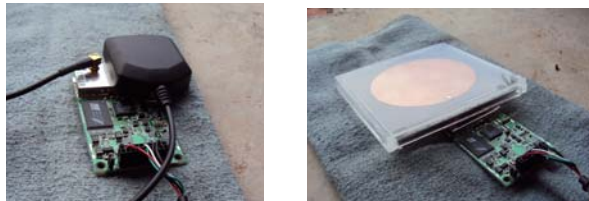
Fig. 15. GPS kit with (a) its original antenna and (b) with the replacement antenna.
