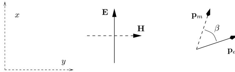
Fig. 6. The directions of the induced electric and magnetic dipole moments in the PEMC sphere are not in general parallel to the incident field vectors. The angle  $\beta$  between the moments depends on  $M$ . This case corresponds to  $M = 1$ .
