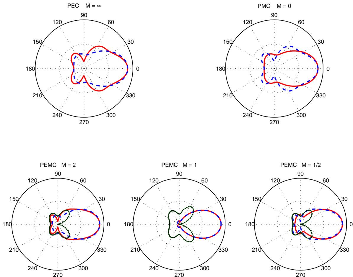
Fig. 13. The scattered far field power pattern of a small reflecting sphere ( $ka = 3$ ) with various values of the  $M$  parameter. Co-polarized in E-plane (solid line) and H-plane (dashed line). The dotted line shows the cross-polarized scattering (the same in both planes). The incident field is coming from the  $180^\circ$  direction.
