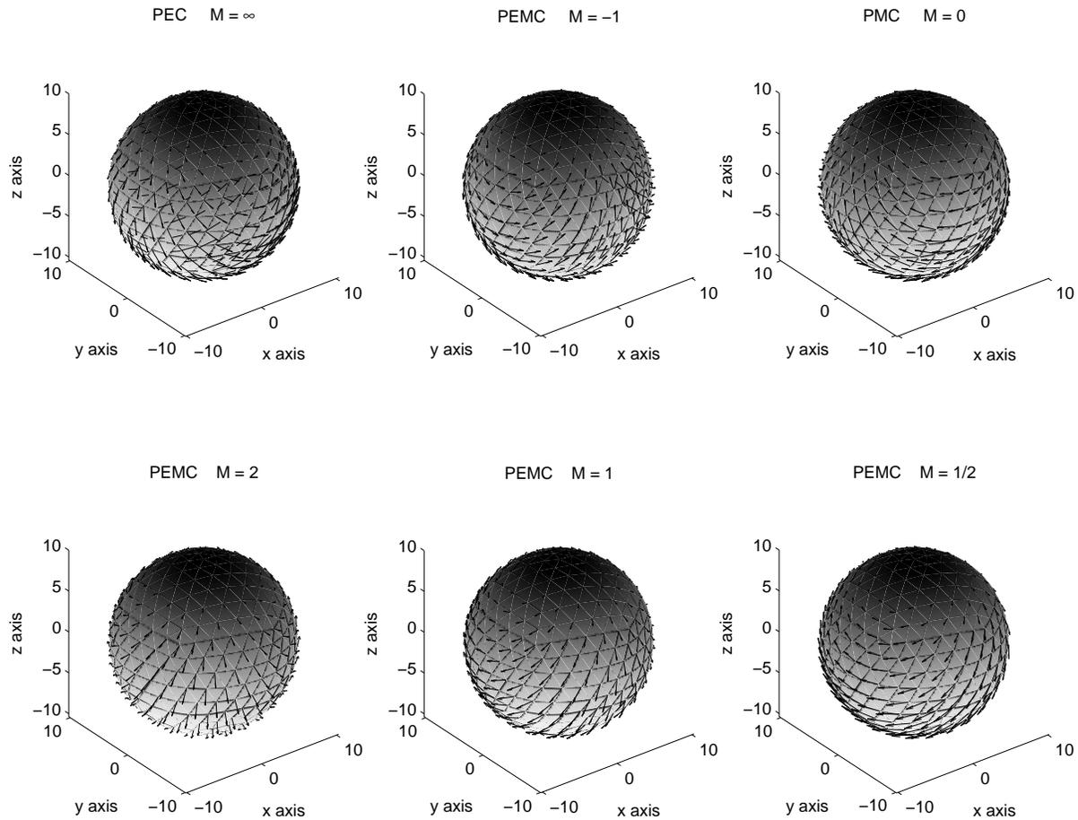
Fig. 15. The scattered far field of the PEMC sphere with varying  $M$  parameters: imaginary part of the electric field. Grayscale shows the amplitude and the arrows display the polarization of the radiated electric field. Incident electric field is parallel to the  $x$  axis. The electrical size of the sphere is  $ka = 1$ .
