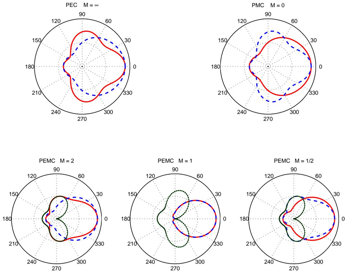
Fig. 12. The scattered far field power pattern of a small reflecting sphere ( $ka = 2$ ) with various values of the  $M$  parameter. Co-polarized in E-plane (solid line) and H-plane (dashed line). The dotted line shows the cross-polarized scattering (the same in both planes). The incident field is coming from the  $180^\circ$  direction.
