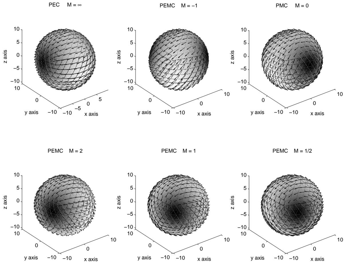
Fig. 14. The scattered far field of the PEMC sphere with varying  $M$  parameters: real part of the electric field. Grayscale shows the amplitude and the arrows display the polarization of the radiated electric field. Incident electric field is parallel to the  $x$  axis. The electrical size of the sphere is  $ka = 1$ .
