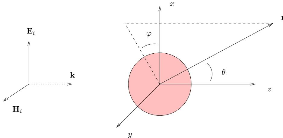
Fig. 1. Geometry of the problem: homogeneous sphere as an obstacle to the incident, linearly  $x$ -polarized electromagnetic wave which is propagating into the  $+z$ -direction. The scattering direction is defined by the angles  $\theta, \varphi$  of the spherical coordinate system.
