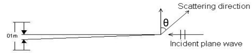
Fig. 10. Wedge geometry considered to compute the Bi-static RCS for a phi-cut = 0^\circ , theta varying from 0^\circ to 180^\circ for an incident plane wave in the direction shown and perpendicularly polarized to the edge of the wedge.
