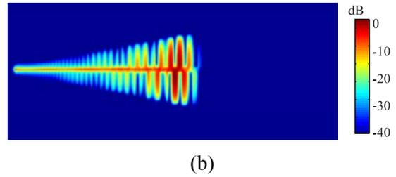
Fig. 5. Surface current density of the proposed PLPA at (a)  $f= 20$  GHz and (b)  $f= 40$  GHz.
