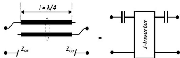
Fig. 2. Equivalent circuit to microstrip coupled lines transformation.
