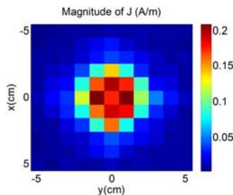
Fig. 9. Variations of the equivalent current ( $|J|$ ) on the PCB plane ( $z = 0$ ) predicted by the proposed model, using the data shown in Fig. 8.
