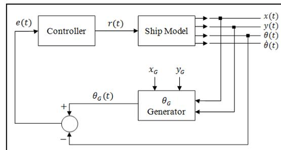
Fig. 5. Block diagram of the PID control system.
