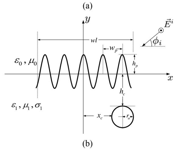
Fig. 2. The medium with (a) flat surface and (b) sinusoidal surface.
