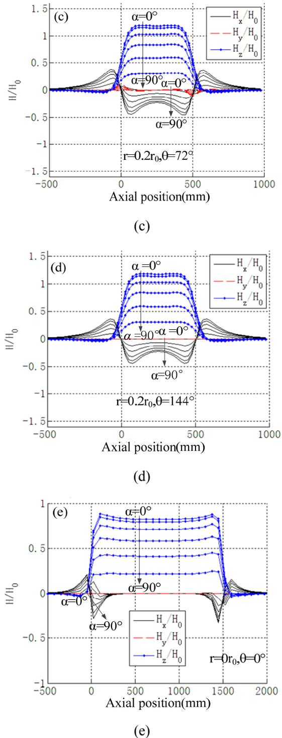
Fig. 6. Magnetic field distributions in different pipes under different directions of magnetization;  $\alpha = 0^\circ, 15^\circ, 30^\circ, 45^\circ, 60^\circ, 75^\circ, 90^\circ$ ;  $r_0 = 100$  mm,  $t = 7$  mm, (a)-(d)  $l_0 = 500$  mm and (e)  $l_0 = 1500$  mm.
