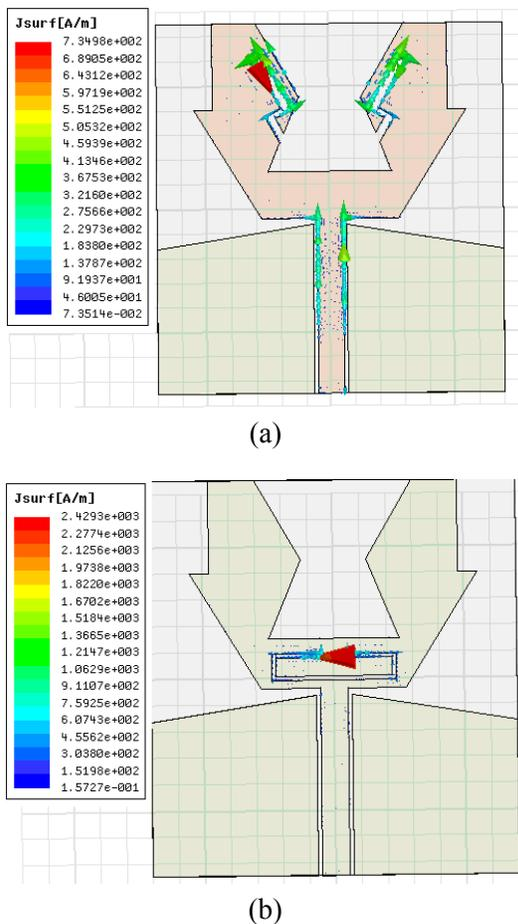
Fig. 2. Current distributions at the notched frequency.
