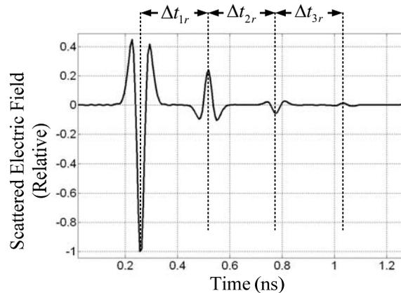
Fig. 7.  $TM_z$  back scattered field from a buried cylindrical PEC object for  $r_a = 0.01$  m,  $h_c = 0.01$  m,  $wl = 2$  m,  $x_c / r_a = 0.0$ ,  $\epsilon_1 = 15 \epsilon_0$  F/m,  $\mu_1 = \mu_0$  H/m,  $\phi_i = \phi_s = 90^\circ$ , and  $\sigma_1 = 0.001$   $Sm^{-1}$ .
