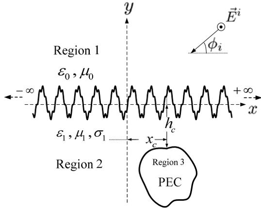
Fig. 1. Geometry of cylindrical object buried inside a lossy half-space with periodic surface.
