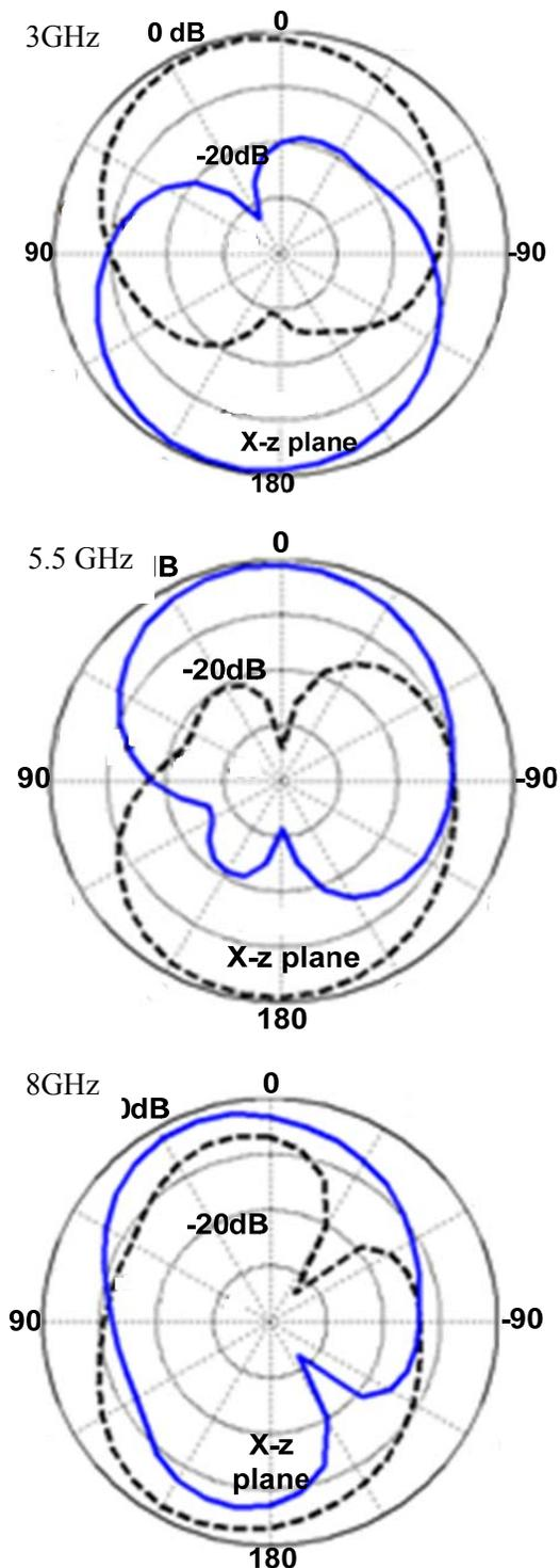
Fig. 5. Measured radiation patterns of the proposed antenna.
