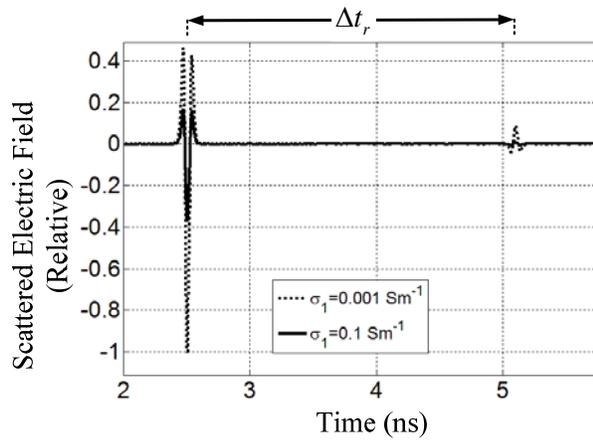
Fig. 9.  $TM_z$  back scattered field from a buried cylindrical PEC object for  $r_a = 0.01$  m,  $h_c = 0.1$  m,  $wl = 2$  m,  $x_c / r_a = 0.0$ ,  $\epsilon_1 = 15 \epsilon_0$  F/m,  $\mu_1 = \mu_0$  H/m,  $\phi_i = \phi_s = 20^\circ$ , and  $\sigma_1 = 0.001$   $Sm^{-1}$ .
