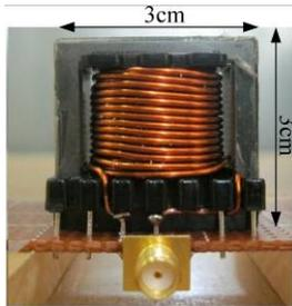
Fig. 7. High frequency inductor.
