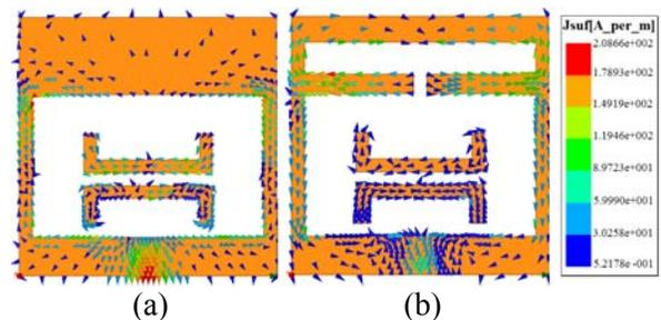
Fig. 5. Simulated surface current distributions on the ground plane for (a) the square antenna with a pair of U-shaped parasitic structures in the ground plane at third resonance frequency (11.15 GHz) and (b) for the proposed antenna at the notch frequency (5.5 GHz).
