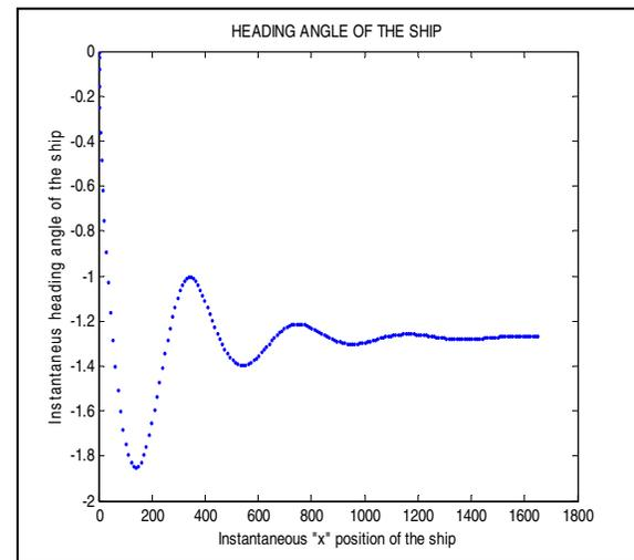
Fig. 7. Instantaneous heading angle of the ship against position 9 km (Case 2).
