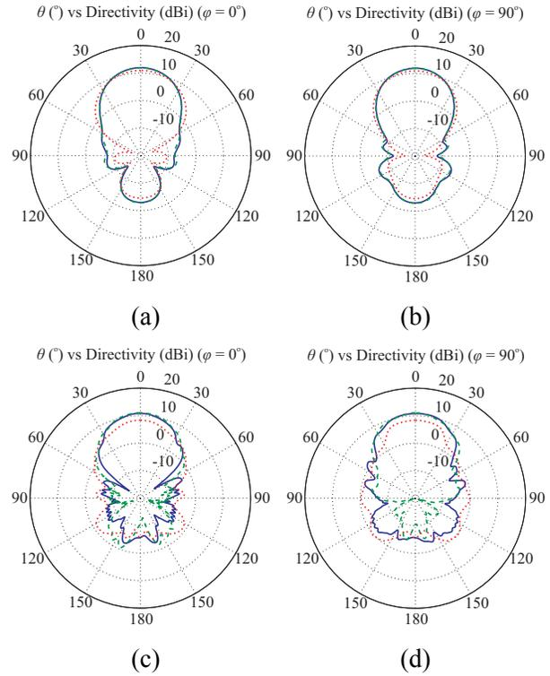
Fig. 13. Radiation patterns of diverse PLPAs with  $c_n = 0.5 (w_n - t_n)$  (blue continuous line),  $c_n = 0.6 (w_n - t_n)$  (green dashed line), and  $c_n = 0.7 (w_n - t_n)$  (red dotted line) at (a), (b)  $f = 20$  GHz, and (c), (d)  $f = 100$  GHz.
