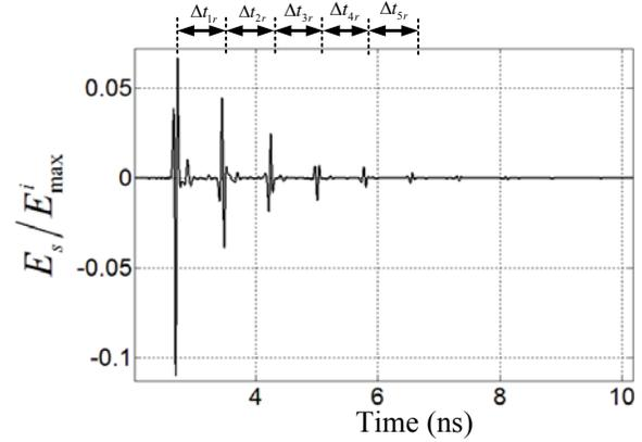
Fig. 10.  $TM_z$  back scattered field from a buried cylindrical PEC object for  $r_a = 0.01$  m,  $h_c = 0.02$  m,  $wl = 2$  m,  $x_c / r_a = 0.0$ ,  $\epsilon_1 = 15 \epsilon_0$  F/m,  $\mu_1 = \mu_0$  H/m,  $\phi_i = \phi_s = 90^\circ$ ,  $w_p = 0.1$  m,  $h_p / w_p = 0.1$ , and  $\sigma_1 = 0.001$   $Sm^{-1}$ .
