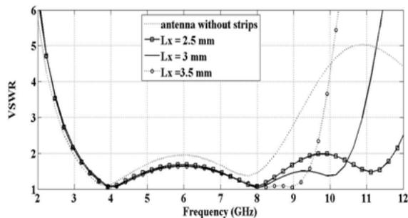
Fig. 3. Simulated VSWR characteristics for different values of  $L_X$  ( $L_Y = 1.2$  mm).
