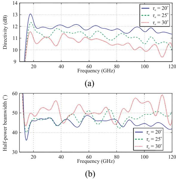
Fig. 6. Performance comparison of several PLPAs for different  $\tau_a$  values, (a) directivity and (b) half-power beamwidth angle.
