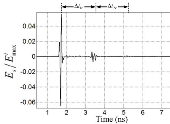
Fig. 11.  $TM_z$  back scattered field from a buried cylindrical PEC object for  $r_a = 0.01$  m,  $h_c = 0.06$  m,  $wl = 2$  m,  $x_c / r_a = 0.0$ ,  $\epsilon_1 = 15 \epsilon_0$  F/m,  $\mu_1 = \mu_0$  H/m,  $\phi_i = \phi_s = 90^\circ$ ,  $w_p = 0.1$  m,  $h_p / w_p = 0.1$ , and  $\sigma_1 = 0.001$   $Sm^{-1}$ .
