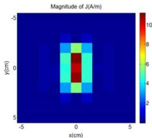
Fig. 13. Variations of the equivalent current ( $|J|$ ) on the PCB plane ( $z = 0$ ) predicted by the proposed model, using the data shown in Fig. 12.
