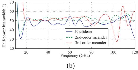
Fig. 14. Comparison between various PLPAs with different elements; (a) directivity and (b) half-power beamwidth.
