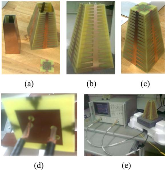
Fig. 8. The volume-confined PLPAs; (a) parts: four-arm radiator, conductive shield, and planar feeding circuit, (b), (c) views of the fabricated prototypes, (d) transmission line cables of the feeding system (internal side), and (e) measurement setup.
