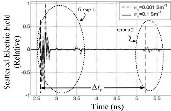
Fig. 12.  $TM_z$  back scattered field from a buried cylindrical PEC object for  $r_a = 0.01$  m,  $h_c = 0.1$  m,  $wl = 2$  m,  $x_c / r_a = 0.0$ ,  $\epsilon_1 = 15 \epsilon_0$  F/m,  $\mu_1 = \mu_0$  H/m,  $\phi_i = \phi_s = 90^\circ$ ,  $w_p = 0.1$  m, and  $h_p/w_p = 0.1$ .
