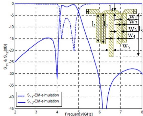
Fig. 9. S-parameters of the compact overlapped BPF (structure 4).
