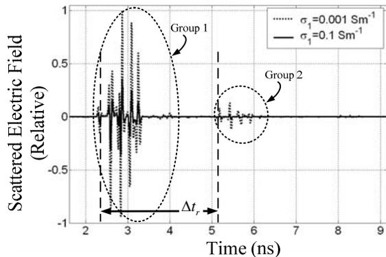
Fig. 13.  $TM_z$  back scattered field from a buried cylindrical PEC object for  $r_a = 0.01$  m,  $h_c = 0.1$  m,  $wl = 2$  m,  $x_c / r_a = 0.0$ ,  $\epsilon_1 = 15 \epsilon_0$  F/m,  $\mu_1 = \mu_0$  H/m,  $\phi_i = \phi_s = 20^\circ$ ,  $w_p = 0.1$  m, and  $h_p/w_p = 0.1$ .
