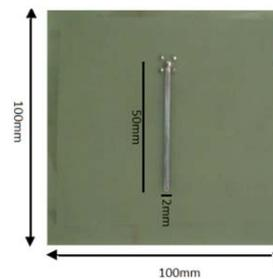
Fig. 11. Microstrip transmission line.
