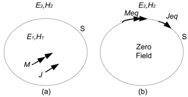
Fig. 2. The electromagnetic equivalence principle; (a) the original problem and (b) the equivalent problem.
