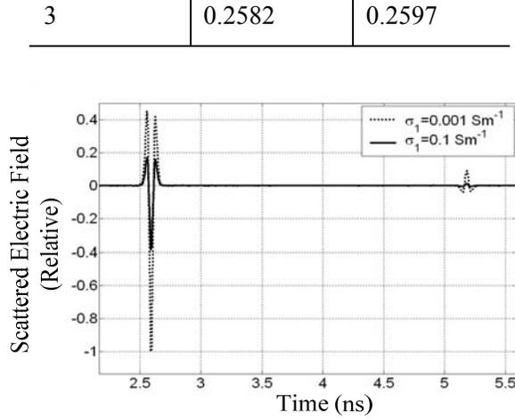
Fig. 8.  $TM_z$  back scattered field from a buried cylindrical PEC object for  $r_a = 0.01$  m,  $h_c = 0.1$  m,  $wl = 2$  m,  $x_c / r_a = 0.0$ ,  $\epsilon_1 = 15 \epsilon_0$  F/m,  $\mu_1 = \mu_0$  H/m, and  $\phi_i = \phi_s = 90^\circ$ .
