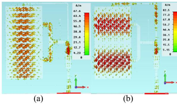
Fig. 4. Surface current distributions of the proposed antenna: (a)  $TM_{10}$  mode when diode 1 is ON and diode 2 is OFF and (b)  $TM_{02}$  mode when diode 1 is OFF and diode 2 is ON.
