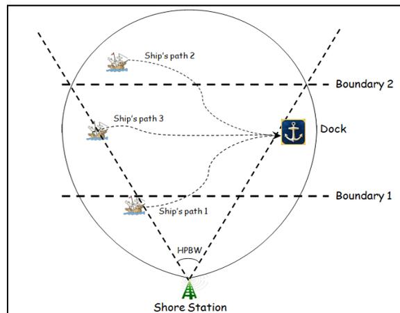
Fig. 3. Ship motion within the half-power beam-width.
