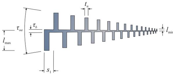
Fig. 1. Geometry of a Euclidean-toothed arm.
