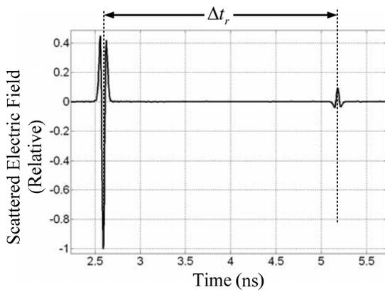
Fig. 6.  $TM_z$  backscattered field from a buried cylindrical PEC object for  $r_a = 0.01$  m,  $h_c = 0.1$  m,  $wl = 2$  m,  $x_c / r_a = 0.0$ ,  $\epsilon_1 = 15 \epsilon_0$  F/m,  $\mu_1 = \mu_0$  H/m,  $\phi_i = \phi_s = 90^\circ$ , and  $\sigma_1 = 0.001$   $Sm^{-1}$ .
