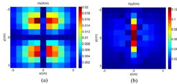
Fig. 12. Variations of the measured tangential magnetic field produced by the microstrip transmission line on the near-field plane ( $h_1 = 10$  mm); (a)  $H_x$  and (b)  $H_y$ .
