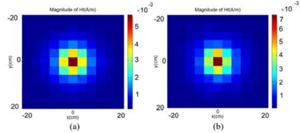
Fig. 10. Variations of the tangential magnetic field ( $\sqrt{H_x^2 + H_y^2}$ ) produced by high frequency inductor on the far-field plane ( $h_2 = 50$  mm); (a) reconstructed and (b) measured results.
