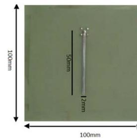
Fig. 11. Microstrip transmission line.
