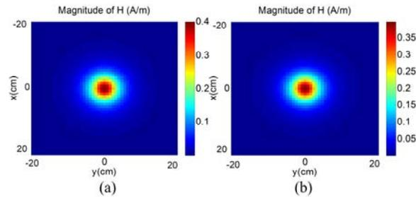
Fig. 6. Variations of the tangential magnetic field ( $\sqrt{H_x^2 + H_y^2}$ ) produced by the electrical loop on the far-field plane ( $h_2 = 50$  mm); (a) theoretical and (b) reconstructed results.
