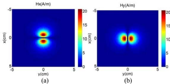
Fig. 4. Variations of the tangential magnetic field produced by the electrical loop on the near-field plane ( $h_1 = 10$  mm); (a)  $H_x$  and (b)  $H_y$ .
