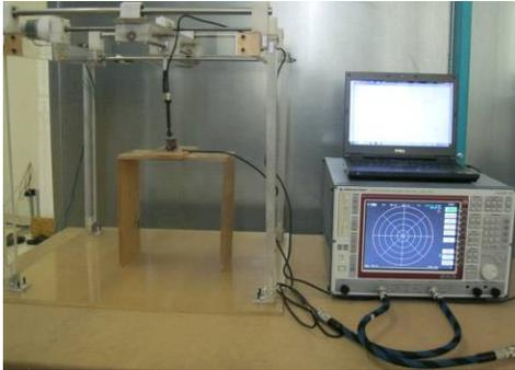
Fig. 3. Experimental setup for magnetic field measurements.
