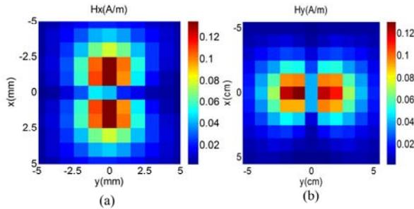
Fig. 8. Variations of the measured tangential magnetic field produced by the high frequency inductor on the near-field plane ( $h_1 = 10$  mm); (a)  $H_x$  and (b)  $H_y$ .
