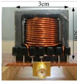
Fig. 7. High frequency inductor.
