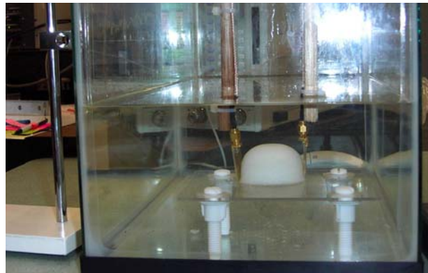
Fig. 4. S -parameter measurement of a breast phantom.
