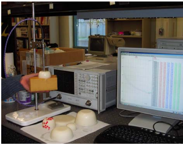
Fig. 6. Measuring the complex permittivity of breast phantoms with Agilent's Dielectric Probe 85070E.
