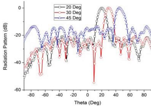
Fig. 5. Optimized radiation patterns using IWO.
