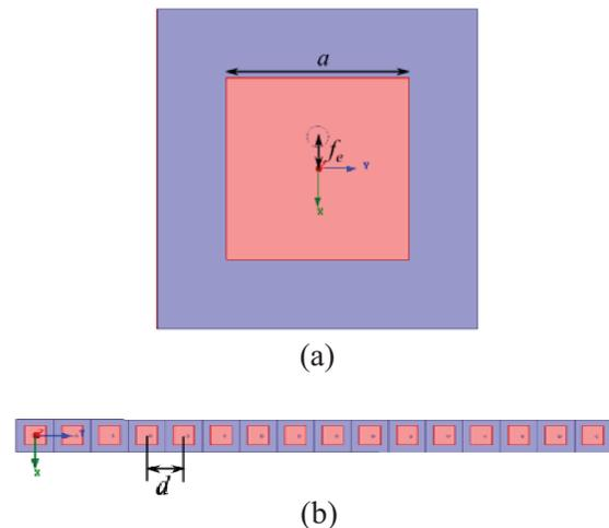
Fig. 2. Configuration of the antenna element and array (a) antenna element and (b) antenna array with substrate characteristics of:  $\epsilon_r = 2.55$ ,  $h = 1$  mm and dimensions:  $a = 8.55$  mm,  $f_e = 1.5$  mm,  $d = 17$  mm.
