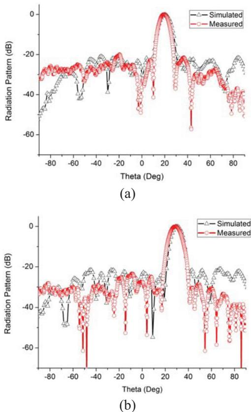
Fig. 8. Measured and simulated radiation pattern (a) beam steering  $20^\circ$  and (b) beam steering  $30^\circ$ .
