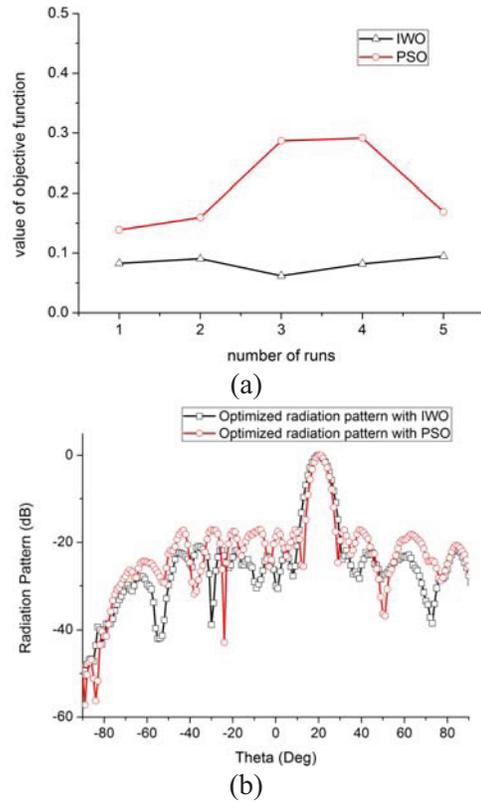
Fig. 4. Performance comparisons of PSO and IWO (a) objective function values obtained from IWO and PSO and (b) radiation pattern optimized by IWO and PSO.
