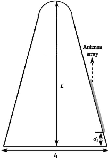
Fig. 3. Configuration of conical carrier and position of the antenna array dimensions:  $L = 1388$  mm,  $l_1 = 400$  mm, and  $d_1 = 65$  mm.
