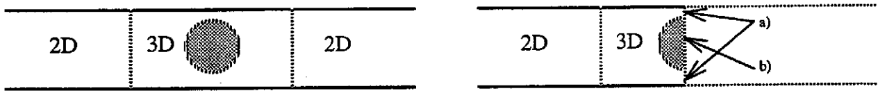
Figure 8: Model of an obstacle in a two-dimensional waveguide without and with symmetries. In region a), an additional wall is introduced. Boundary b) is only needed in certain cases.
