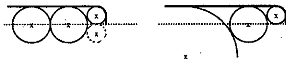
Figure 7: Dependence between multipole and its mirror image, and non-dependence for multipoles symmetrized according to Equation 6. The “forbidden” regions are indicated by the spheres. The positions of the poles are no longer limited to the inside of the conducting plane.
