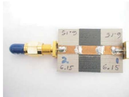
Fig. 8. Snapshot of microstrip transmission line setup for experimental measurements.
