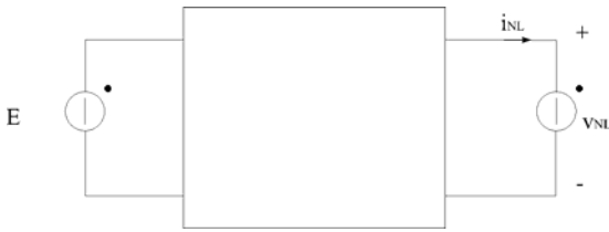
Fig. 2b. Application of the substitution's theorem.
