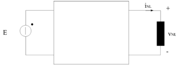
Fig. 2a. Circuit with a nonlinear load.
