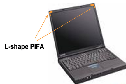
Fig. 2. Proposed antenna locations inside of a laptop computer.
