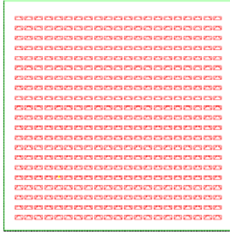
Fig. 1. Illustration of 21 \times 21 rectangular waveguides. The picture symbolically shows the TE_{10} mode excitation in each waveguide.
