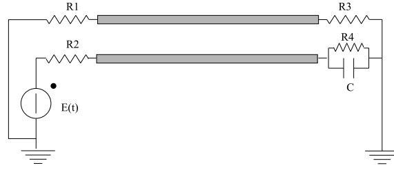
Figure 8: Double conductor nonuniform line with capacitive load
