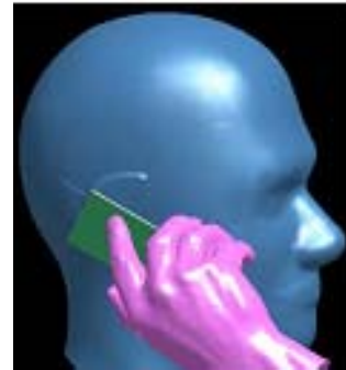
Fig. 1. Complete model used for simulation including handset and SAM phantom head.
