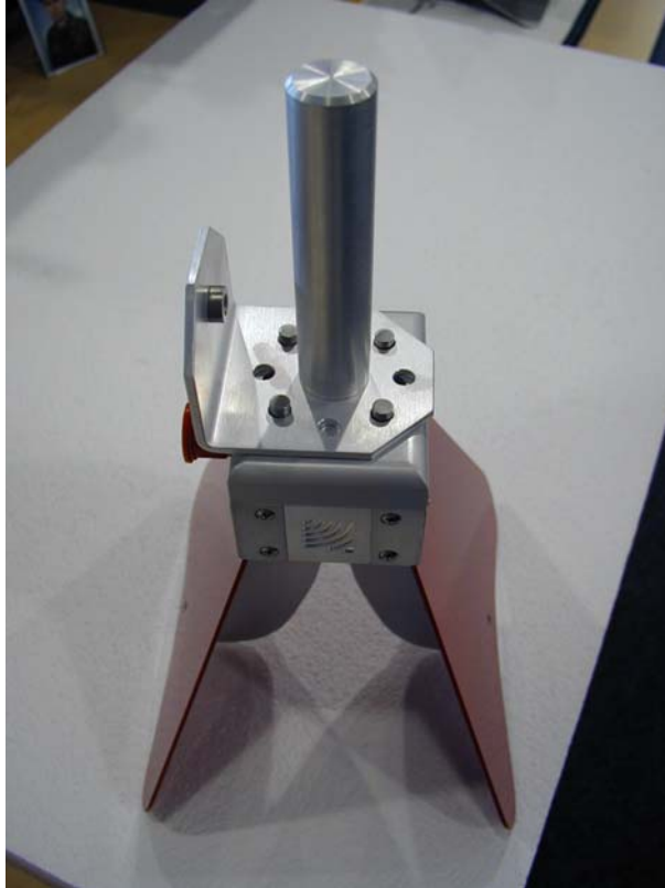
Figure 13. The new horn in showing the extended top and bottom that allows for storing it facing down.
