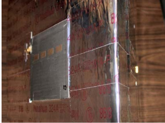
Figure 7. Actual array(s) placed on a slanted (wedge) ground plane.
