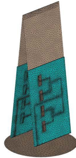
Figure 12. FEKO wedge model with a metallic back plate.
