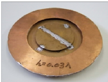
Fig. 9. Photograph of the fabricated top-loaded triangular antenna with folded rim at h = 0.03\lambda .
