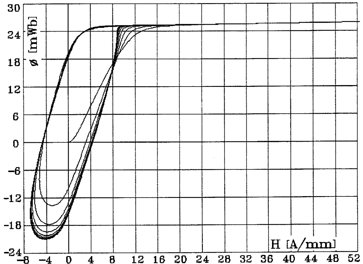
Fig. 11. Core magnetizing loops
