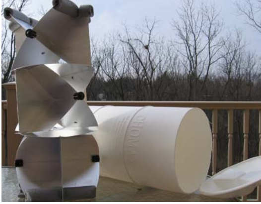
Fig. 2. Photograph of the Echomax 230 reflector and its plastic cylindrical cover.
