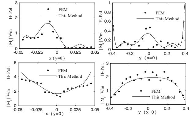
Fig. 5. Comparison between magnetic current of DIES and FEM for the crack of Fig. 1 with  $a = 0.1\lambda$ ,  $b = 0.8\lambda$ ,  $c = 0.25\lambda$ ,  $h = 0.1\lambda$ ,  $\epsilon_2 = 3.2 - 0.1j$ ,  $\epsilon_3 = 1$  for horizontal polarizations (H-Polarization) when  $\phi_i = 0^\circ$  and  $\theta_i = 45^\circ$ .
