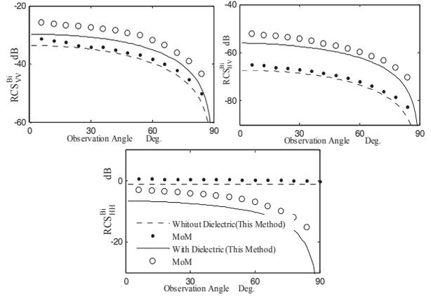
Fig. 8.  $RCS^{bi}$  of the crack in Fig. 1 at various observation angles  $\theta_o$  with  $a=0.1\lambda$ ,  $b=0.8\lambda$ ,  $c=0.25\lambda$ ,  $h=0.1\lambda$ ,  $\epsilon_2=3.2-0.1j$  and  $\epsilon_3=1$  at  $\phi_i=0^\circ$  and  $\theta_i=45^\circ$ .
