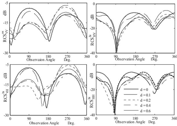
Fig. 10.  $RCS^{bi}$  of the crack in Fig. 1 versus observation angles  $\phi_o$  for different dielectric thicknesses where  $a=0.2\lambda$ ,  $b=1\lambda$ ,  $c=0.25\lambda$ ,  $h=0.1\lambda$ ,  $\epsilon_2=2.5-j0.05$  and  $\epsilon_3=1$  at  $\phi_i=45^\circ$  and  $\theta_i=30^\circ$ .
