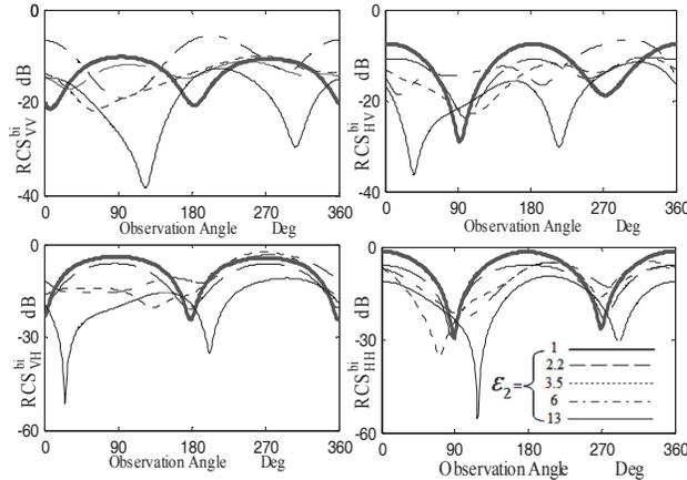
Fig. 9.  $RCS^{bi}$  of the crack in Fig. 1 versus observation angles  $\phi_o$  or materials of table 1 where  $a=0.2\lambda$ ,  $b=1\lambda$ ,  $c=0.25\lambda$ ,  $h=0.1\lambda$  and  $\epsilon_3=1$  at  $\phi_i=30^\circ$  and  $\theta_i=30^\circ$ .
