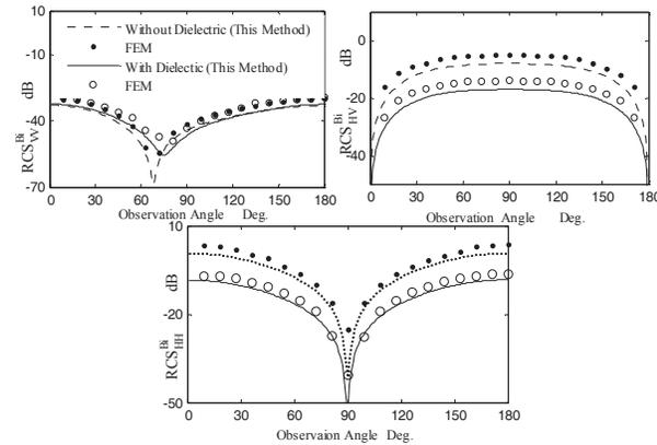
Fig. 7. Bistatic radar cross sections ( $RCS^{bi}$ ) of the crack in Fig. 1 at various observation angles  $\phi_o$  with  $a=0.1\lambda$ ,  $b=0.8\lambda$ ,  $c=0.25\lambda$ ,  $h=0.1\lambda$ ,  $\epsilon_2=3.2-0.1j$  and  $\epsilon_3=1$  at  $\phi_i=0^\circ$ .
