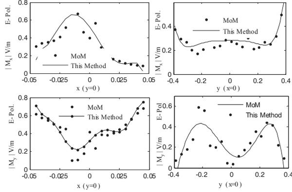
Fig. 6. Comparison between magnetic current of DIES and MoM for the crack of Fig. 1 with:  $a=0.1\lambda$ ,  $b=0.8\lambda$ ,  $c=0.25\lambda$ ,  $h=0.1\lambda$ ,  $\epsilon_2=3.2-0.1j$  and  $\epsilon_3=1$  for vertical polarizations (E-Polarization) at  $\phi_i=0^\circ$  and  $\theta_i=45^\circ$ .
