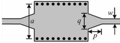
Fig. 7. Transmission SIW to microstrip lines.
