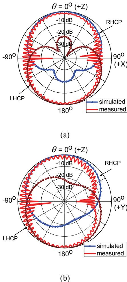
Fig. 11. Measured and simulated normalized RHCP/LHCP radiation patterns of the proposed antenna at 915 MHz. (a) x-z; (b) y-z plane.
