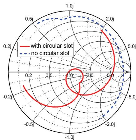
Fig. 3. Simulated Smith Chart for different circular slot radii ( $R_3$ ).
