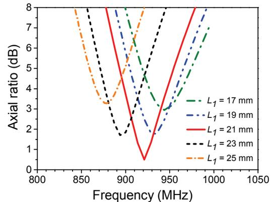
Fig. 5. Simulated axial ratio for different lengths of meandered slot section ( $L_1$ ).
