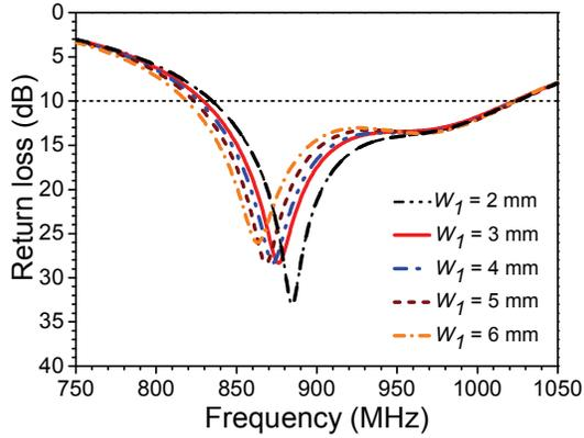
Fig. 6. Simulated return loss for different widths of meandered slot section ( $W_1$ ).
