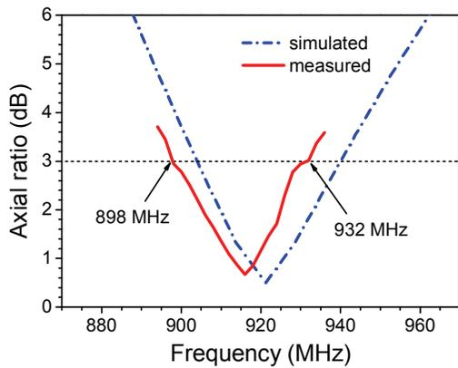
Fig. 10. Measured and simulated axial ratios of the proposed antenna.
