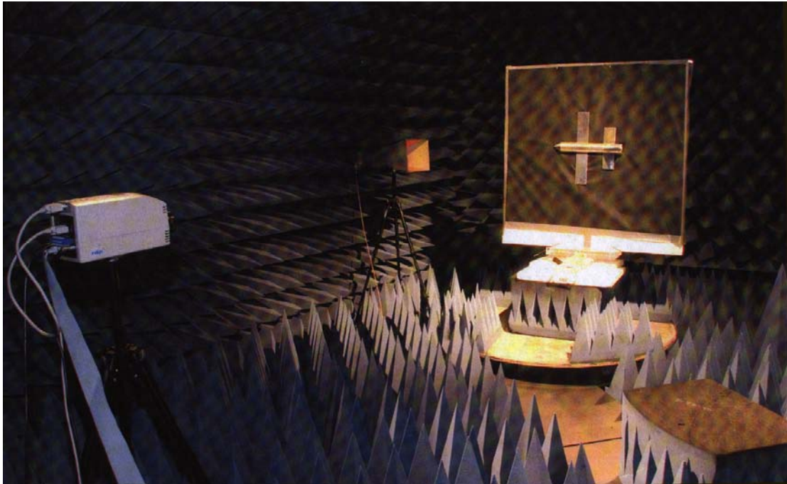
Figure 1. Anechoic Chamber and Test Article Setup with Horn Antenna and IR Camera
