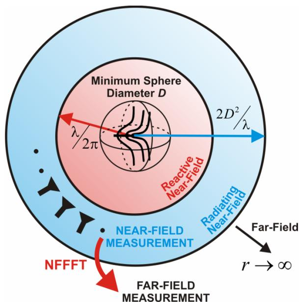
Fig. 1. Antenna field regions and measurement setup.
