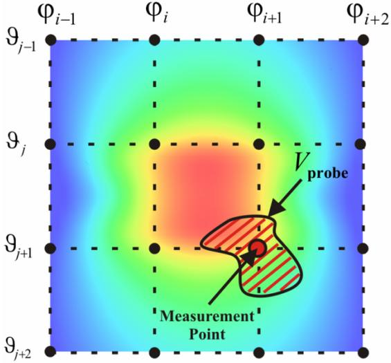
Fig. 2. Probe weighting effect in electric near-field measurement.
