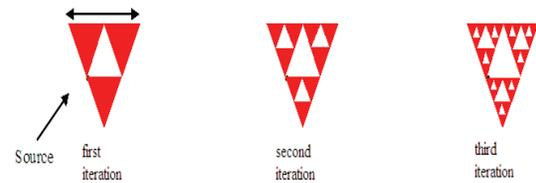
Fig. 8. First three iterations of Sierpinski antenna.
