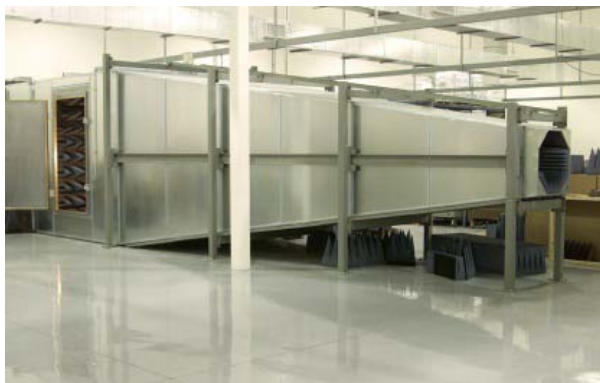
Fig. 1. A typical tapered anechoic chamber.
