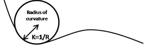
Fig. 3. Radius of curvature of a wire.
